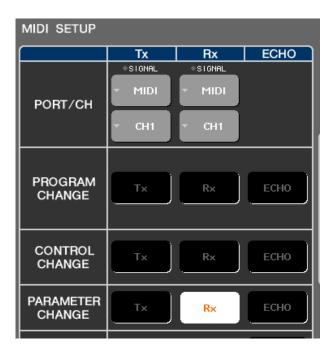
Configure the M7CL so that it can receive MIDI channel 1 signals from the external device through the MIDI port.
