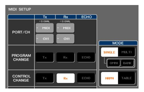
Configure the M7CL so that it can receive MIDI channel 1 signals from the external device through the MIDI port.
