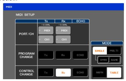
2. Configure the settings so that MIDI channel 1 signals can be received from the external device through the M7CL MIDI port. You can use a different MIDI channel as long as the channels on the transmitting device and the receiving device are the same.
