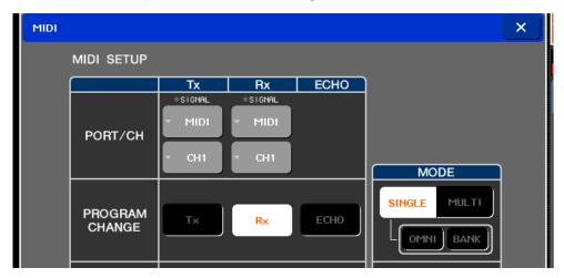
Configure the M7CL so that it can receive MIDI channel 1 signals from the external device through the MIDI port.
