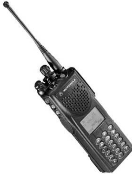
Figure 4.1 A photo illustration of a Motorola Inc. XTS 3500 portable radio. It is identical in appearance to the XTS 3000, except it has a purple keypad and a different model number sticker above the speaker-grill.
