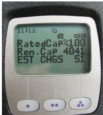
Figure 6.6 A photo illustration of a Motorola XTS 5000™ displaying IMPRES™ battery data via the BATT soft-menu. In addition to this data, note the battery gauge in the upper-right display.
