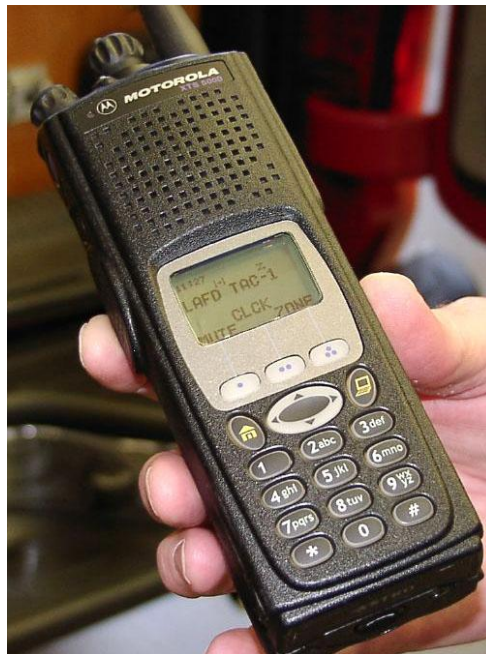
Figure 6.1 Photo illustration of a Motorola Inc. XTS 5000™ in a model III configuration.
