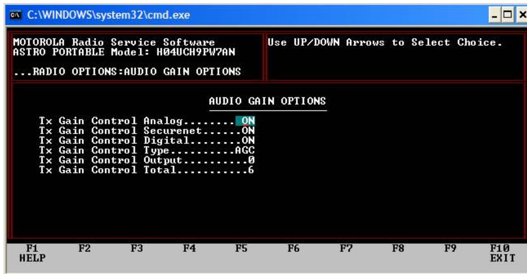
Figure 9.1 Recommended settings for optimized subscriber AGC operation in ASTRO™ RSS.
