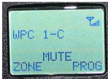
Figure 11.9 A Motorola Inc. XTS 3000 with R06.xx.xx host firmware installed. Note the signal meter in the upper-right display.
