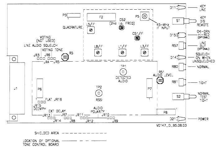
Figure 7-5 IF Board Controls and Indicators
