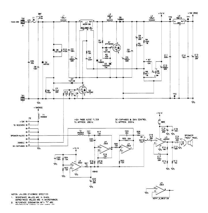
Figure 10-5 PS/A Board Schematic
