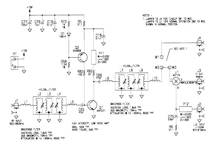
Figure 10-3 Front End Schematic
