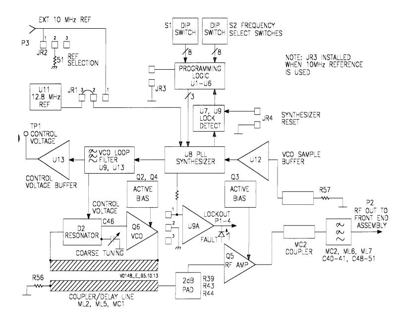
Figure 6-1 Synthesizer Functional Diagram
