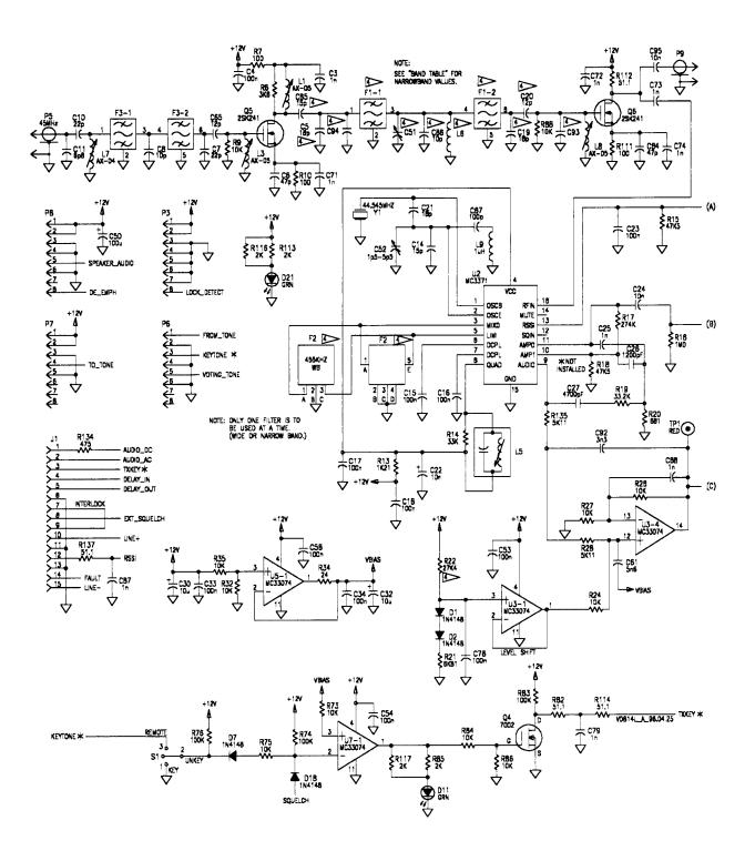
Figure 10-2 IF Audio Board Schematic
