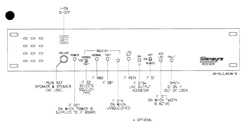
Figure 5-1 Front-Panel Controls and Indicators
