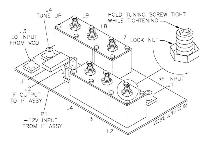
Figure 7-4 RF Assembly - Adjustments
