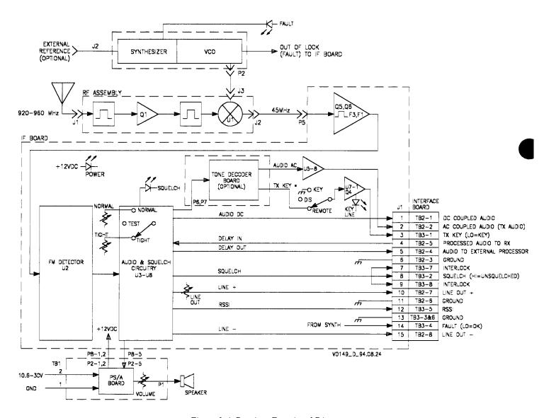
Figure 3-4 Receiver Functional Diagram
