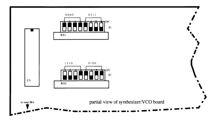
Figure 7-3 Programming Synthesizer Frequency
