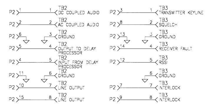
Figure 10-1 Interface Board 265-0305-002 Assembly and Schematic
