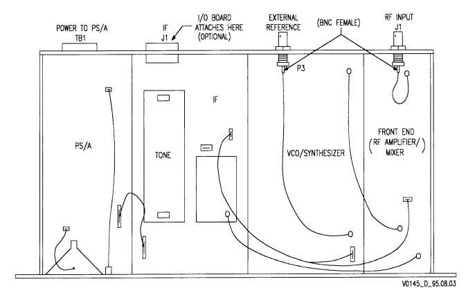
Figure 3-3 Top View of Internal Assemblies
