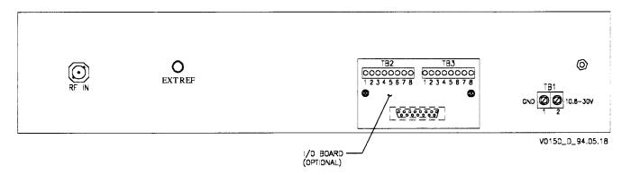
Figure 3-2 Receiver Rear View
