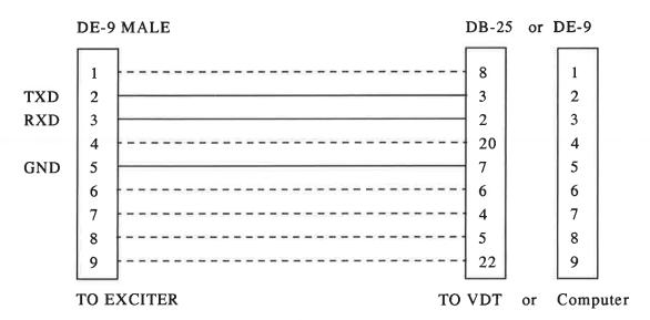
Note: The solid lines show the conductors necessary for the exciter and VDT (or computer) to communicate. The dotted lines show the rest of the conductors in the standard cables.
