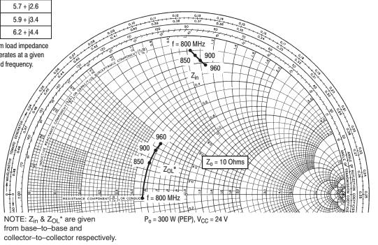
Figure 8. Series Equivalent Input/Output Impedances
