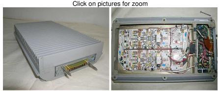
Connector end, unmodified PA Inside unmodified PA
