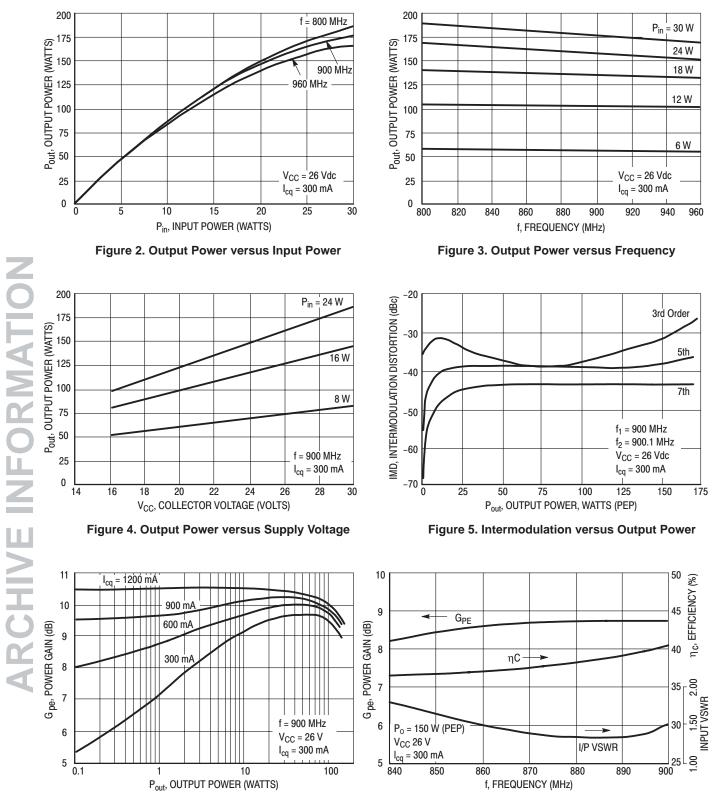
Figure 6. Power Gain versus Output Power
