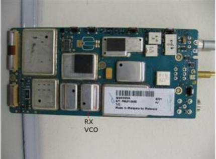
Now comes the hard part: removing the RX VCO shield or can. Using special purpose hot air tools would be ideal, but since I don't have these at my disposal, I opted for using a Dremel tool to cut off the top of the can to access the RX VCO components.
