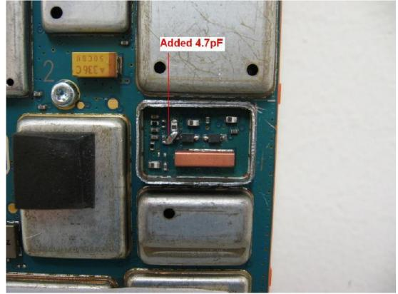
To solder in this tiny SMD chip capacitor will require a low wattage and very fine tipped soldering iron, and some very fine solder. Don't fool yourself, a standard size soldering iron tip simply will not do. A magnifying lens to assist in seeing the area you're soldering will be a great help... I use a loupe or magnifying eye monocle myself. Once soldered in, you'll have achieved the following circuit mods, as seen in this schematic:
