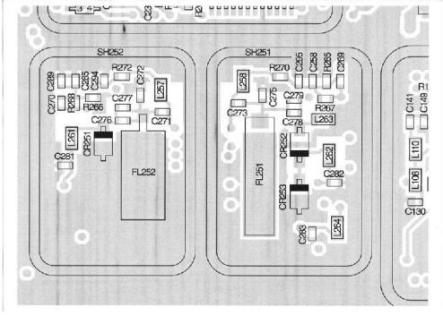
Note that even though C278 is shown as being present, in actual production radios, this component is missing. It is this position that you'll be soldering a 4.7pF SMD chip capacitor. Obtaining a 4.7pF chip cap of the right size (0402) would be useful, but if all you can obtain is the next size up (0603) then you can still make use of this, as the following photo shows:
