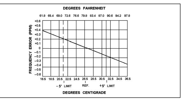
Figure 7 - Frequency Characteristics Vs. Temperature
