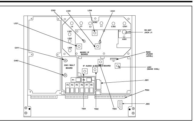
Figure 5 - Test Points And Alignment Controls
