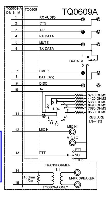
Rev-A: Transformer and load added to test M-RK radios. DB15M connector added and test cable for M-PD/M-PA families changed to have a DB15-F connector on the cable rather wired into the test box. Box changed to TQ0609-A.
