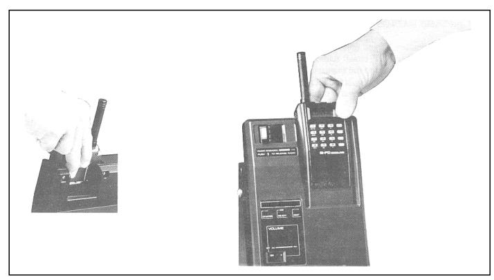
Figure 2 - Inserting And Removing Portable Radio Unit
