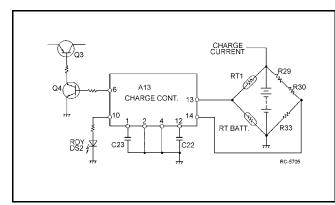
Figure 3 - Simplified Temperature Cut Off Circuit
