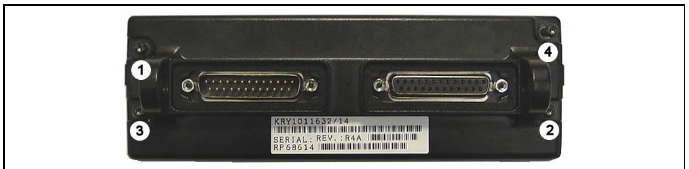
Figure 4-14: Rear Cover Torque Sequence (Remote)
