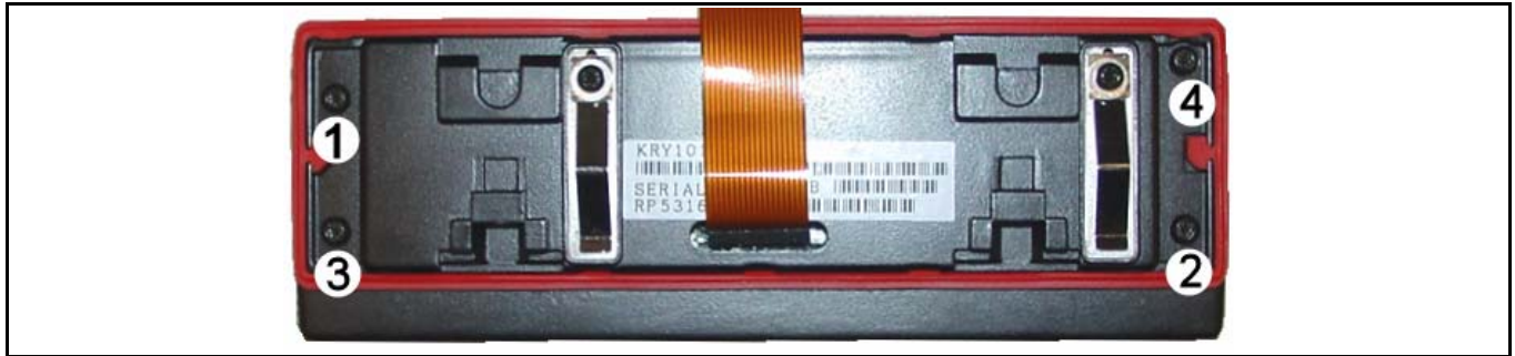
Figure 4-12: Rear Cover Torque Sequence (Local)
