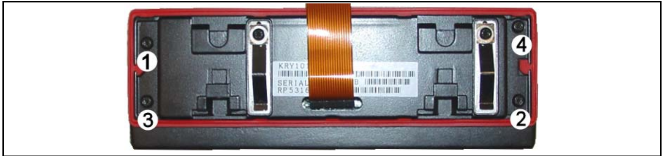
Figure 4-12: Rear Cover Torque Sequence (Local)
