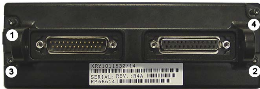
Figure 4-14: Rear Cover Torque Sequence (Remote)
