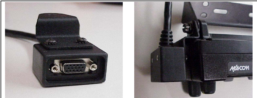
Figure 31: DB15 connector mounted on Control Unit Pigtail Bracket and Pigtail Bracket installed on Control Unit
