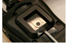
2) Very slowly and carefully rotate the screwdriver to arch the Woofer Port Insert while holding it in place
