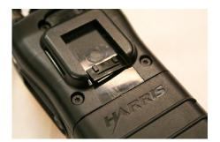
5) Arch the insert by rotating the screwdriver, then guide the other end into the woofer port.
