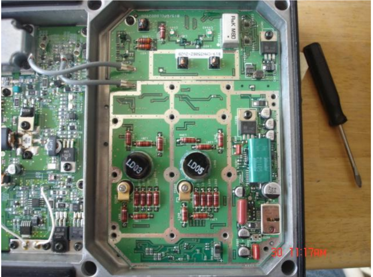
Figure 4. Receiver synthesizer covers and board removal.
