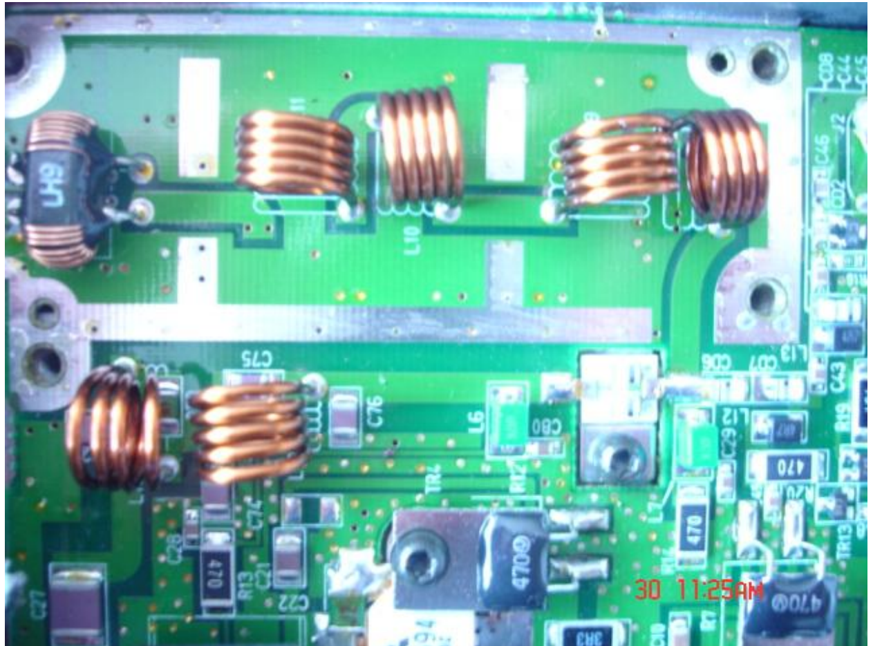
FIGURE 10. transmitter tuning. L18 and L19 lower left. L8 thru L11 upper center.
