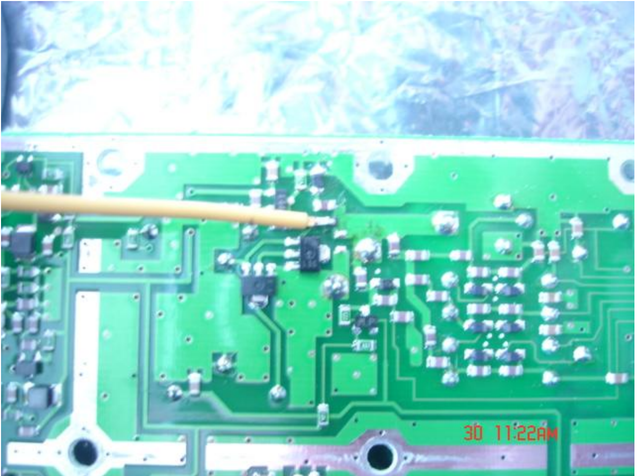
FIGURE 6. Location of C285 on the transmit VCO.
