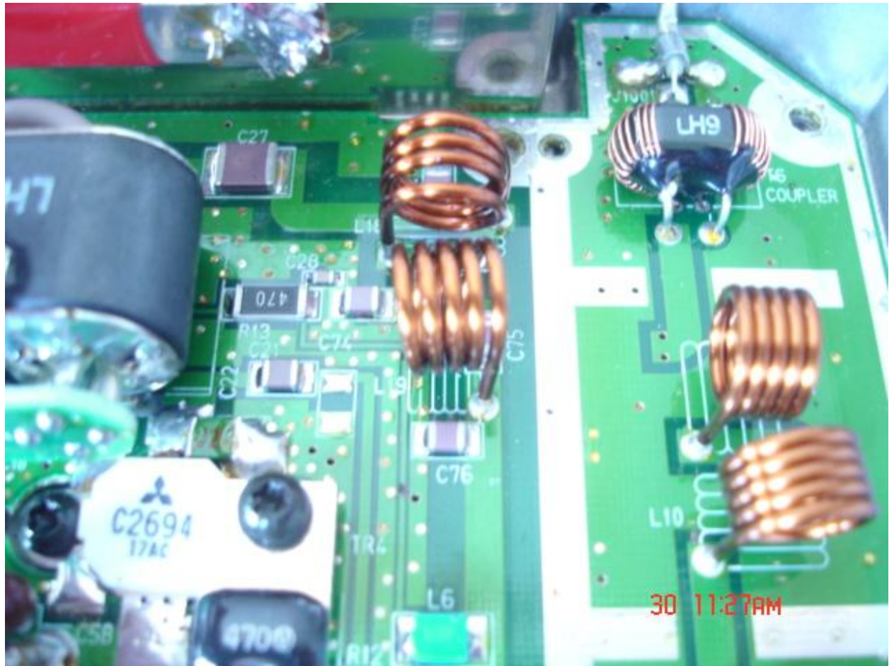
Figure 11. Inductors L18 and L19 upper center. L10 and L11 to the right.
