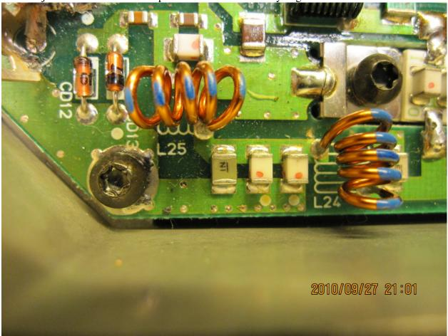
Figure 7. Receiver ¼ wave line. Presetting of L24 end turns at 1 wire spacing and the middle turns at ½ wire spacing. Set L25's end turns at 2 wire spacing and the middle turns at 1 wire spacing.
