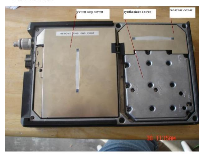
Using the #10 TORX bit remove all screws and set the solid synthesizer cover aside. Remove the Receiver Synthesizer board from the chassis.
