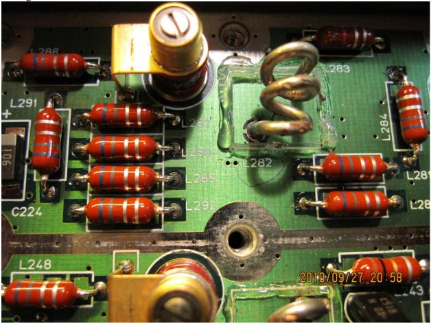
FIGUERE 2. L282 Spread TX VCO coil and adjust TX tuning capacitor CV280 for transmit VCO lock.
