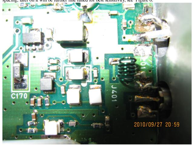
FIGURE 6. RX input inductor, L01 (L401) preset.
