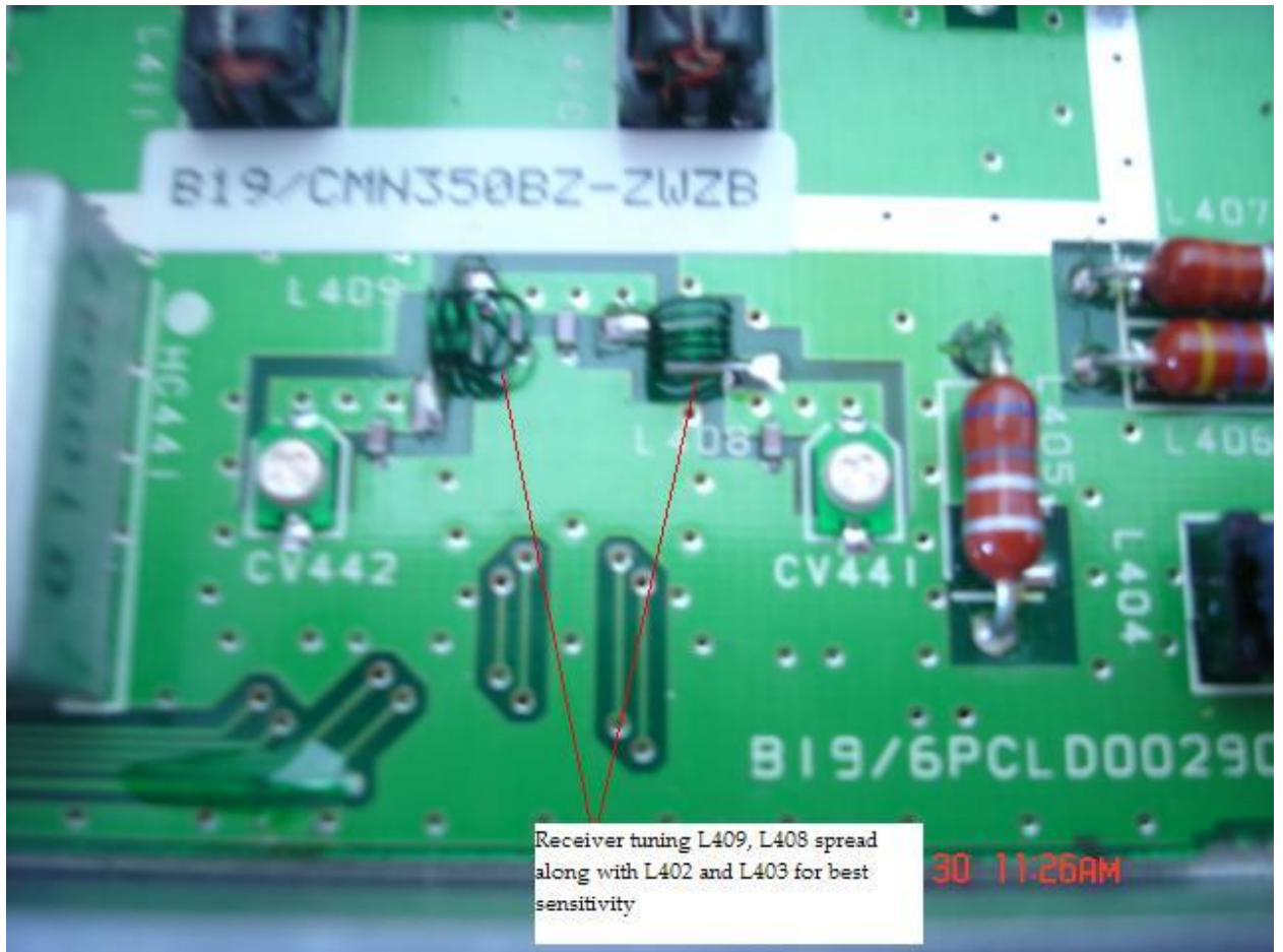
Figure 9, receiver tuning inductors L408 and L409.
