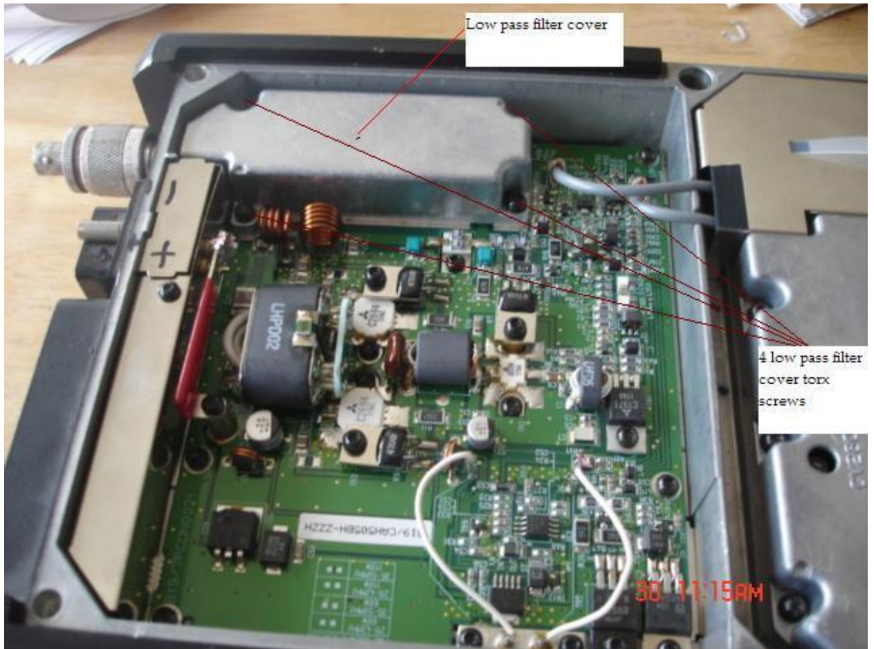
Figure 3. remove the cover at the upper TOP to access the low pass filter inductors.
