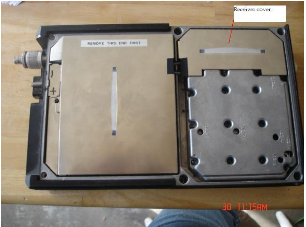
Figure 2, again remove the small cover over the receiver section on the upper right of the board.
