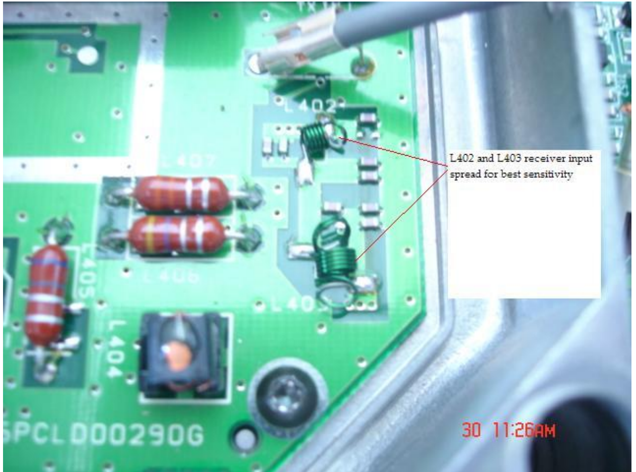
Figure 8, Receiver tuning L402 and L403.
