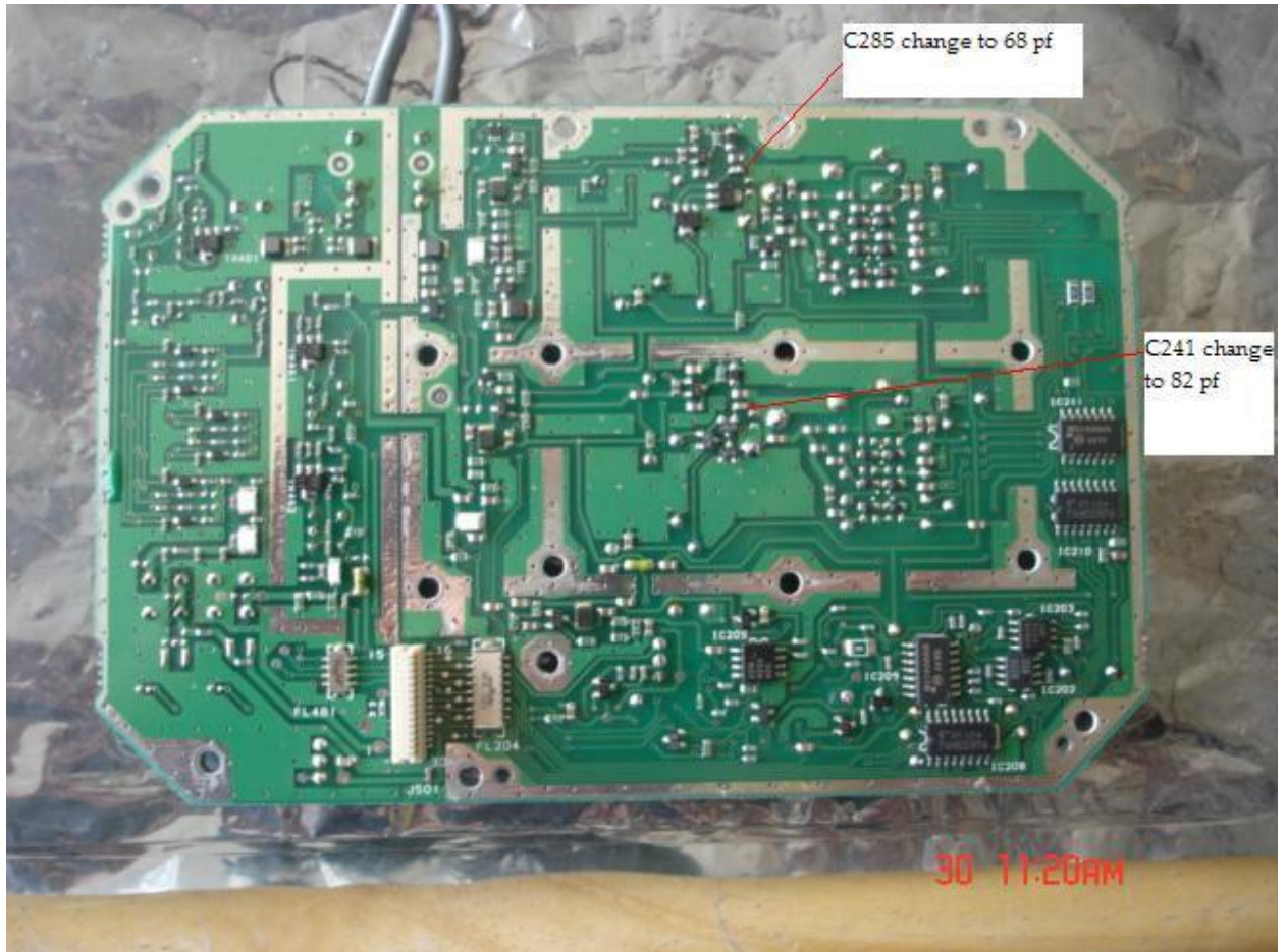
Figure 5. receiver/synthesizer board back side components. C285 is near the top just right of center and C241 is vertically in line with it but near the board center.
