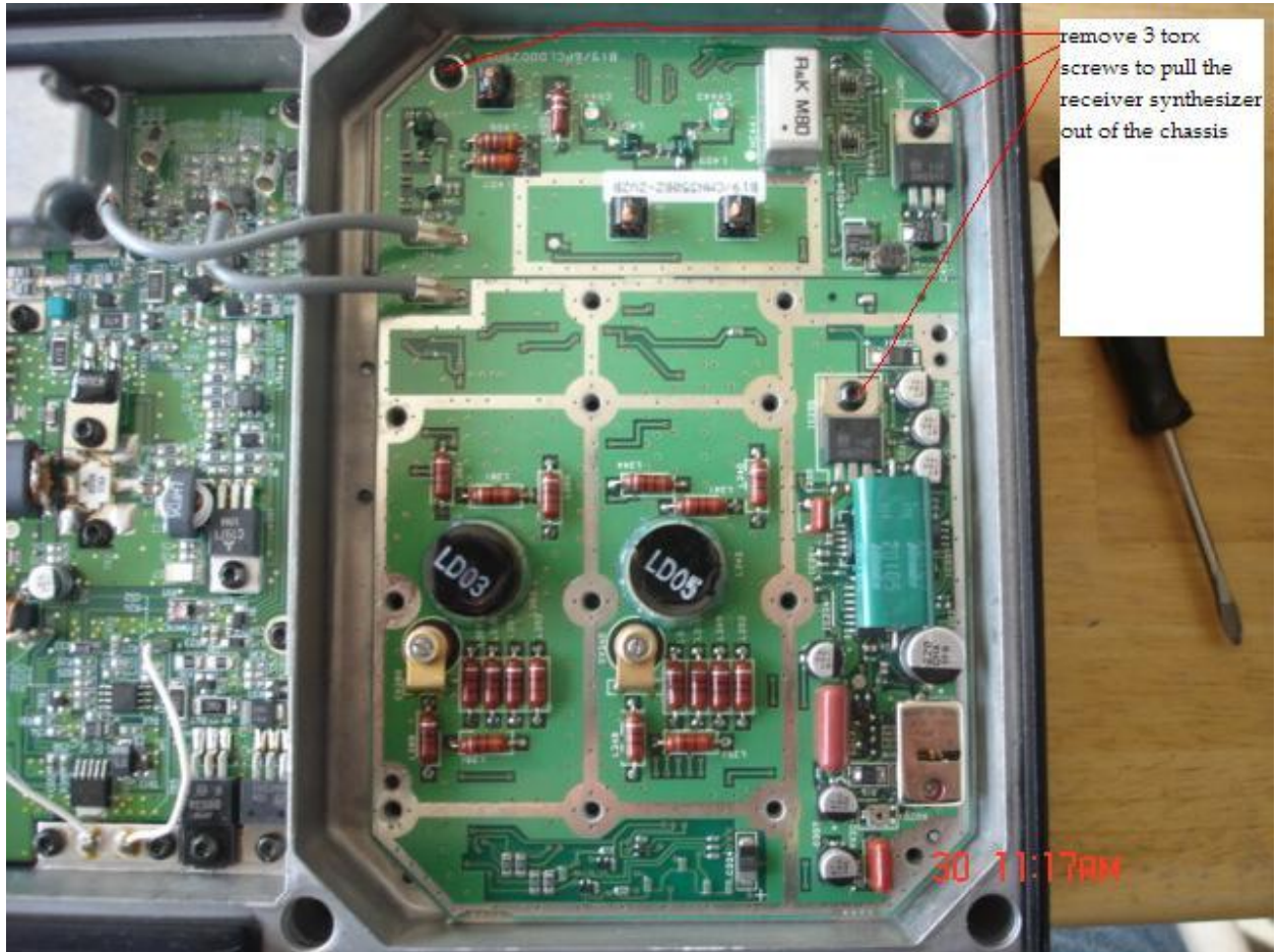
Figure 4. Receiver synthesizer covers and board removal.
