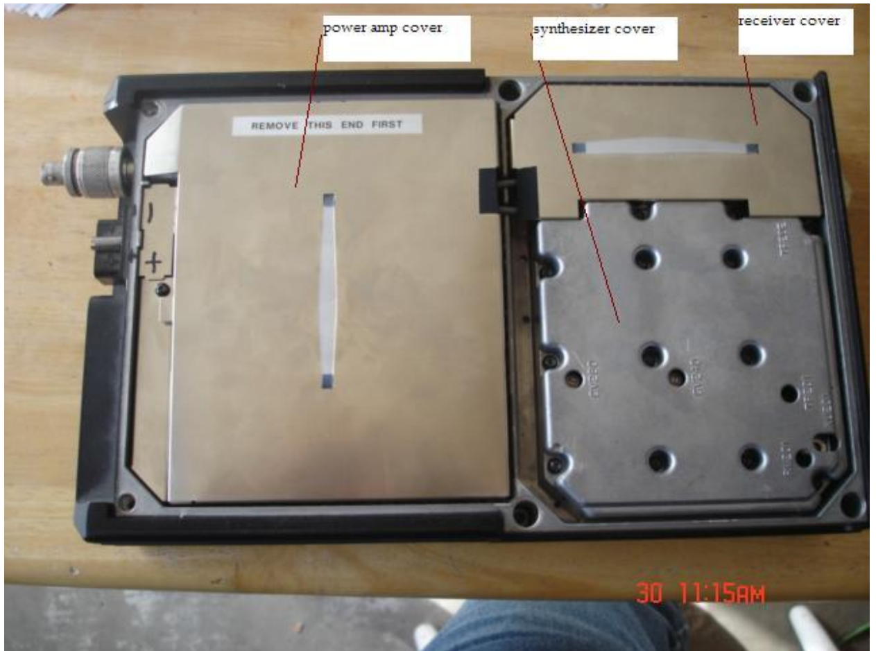
Figure 2. remove the Shield on the left side that is over the power amplifier board.
