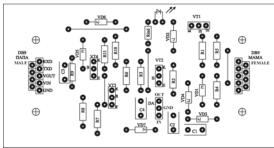
Please note, that R12 is omitted on the PCB, Rind resistor and a LED are added between the DA1 output and the ground to indicate the power. You can omit R12, Rind and a LED, the cirquit will work. Some words are in Russian, the most significant words are translated. The recommended value of Rind is 4.3 kOhm to minimize the current consumption.
