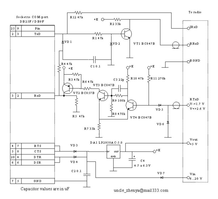
Connection cirquits (jacks for mobile radios are shown as they are plugged into sockets)
