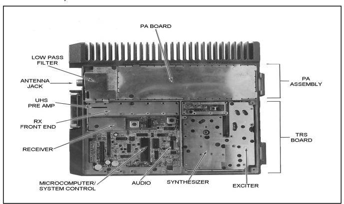
Figure 1 - Typical Module Layout
