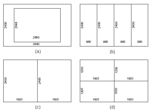
Figure 4. Input modes for Model T221. (a) singlel-screen with 1DVI input, example shown of 1280x1024 input with 2x replication. (b) 4-stripe with 4 DVI inputs. (c) 2-stripe with 2 DVI inputs. (d) quad tile with 4 DVI inputs
