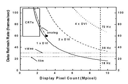
Figure 5. Maximum data refresh rates versus display pixel count for different numbers of DVI inputs.
