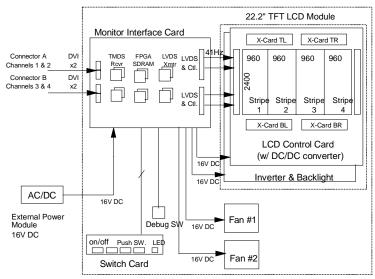
Figure 3. Block diagram of drive electronics.
