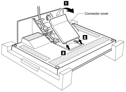
4. Unhook the digital signal cable from the cable hook and lift it up to store the connector tool in the rear compartment of the monitor.
