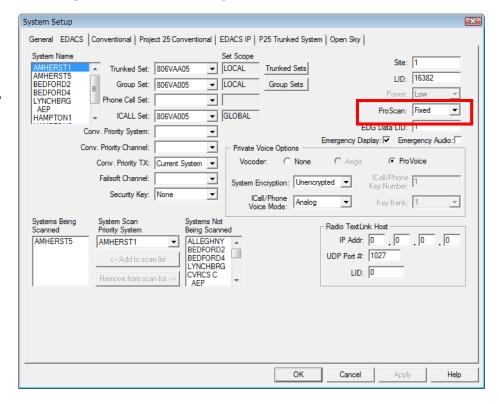
stream, originating from the radio system's IMC, a radio in FIXED ProScan mode <u>ignores</u> this additional data.
