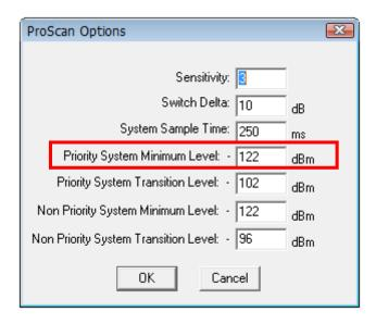
Type a numeric value in the range from -60 to -122 dBm.
