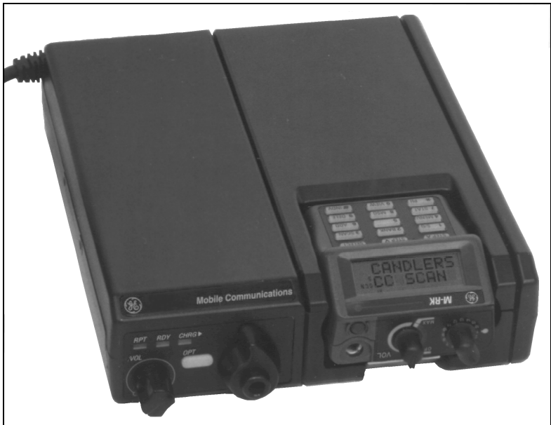
Figure 2 - Charger With M-RK II Personal Radio Inserted (Antenna Removed For Photo Only).
