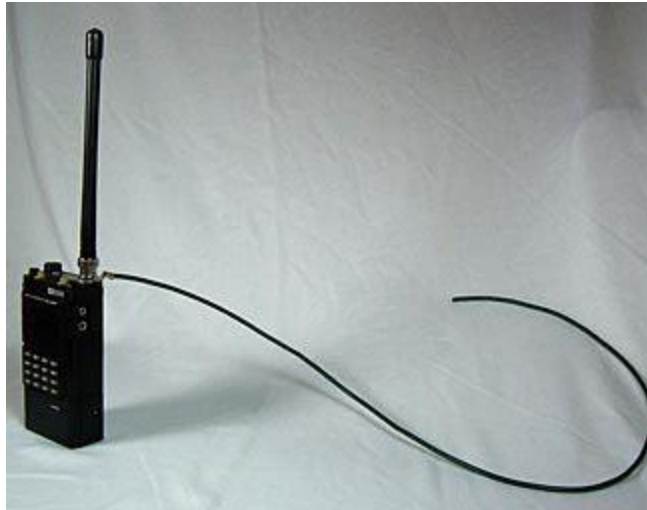
Adding a simple piece of wire to your walkie-talkie could double its range.
