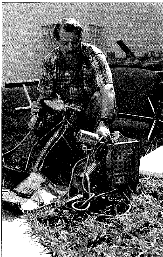
Joel Kandel, KI4T, inspects what's left of a Dade County repeater following Andrew. The repeater took a 1000-foot fall when it came down during the storm along with the 2000-foot-high Channel 6 TV tower. (photo courtesy of KI4T)
