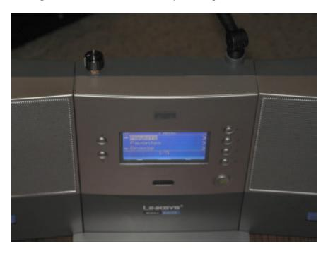
I mounted the new contrast potentiometer on the top of the center unit on the left side. I'd like to say that I chose this spot for its artistic balance with the antenna; but in reality the case interior presents few options to mount readily-available potentiometers.
