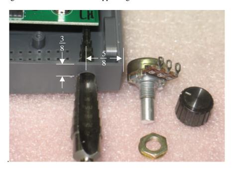
The potentiometer I used is slightly different from the Radio Shack one but is almost the same size. Remove the rear switch and metal barrel from the RS pot to get it to fit.
