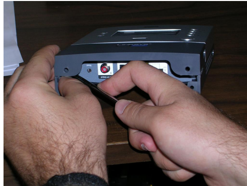
Figure 6: Disengaging the Plastic Retaining Clips
