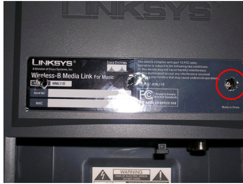
Figure 4: Locating the Hidden Screw Hole on the WMLS11B
